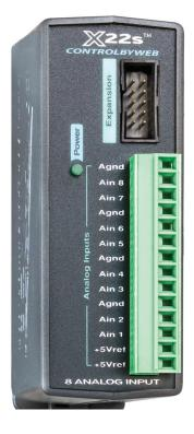
The X-22s has eight precision analog inputs that can be configured for various voltage ranges and 4-20mA sensors.
