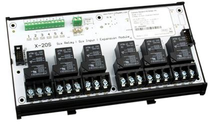
The X-20s<sup>™</sup> expansion module is used with the X-600M controller. The X-20s has six, high-current relays, each with Form-C contacts (SPDT) and six, optically-isolated digital inputs. A screw terminal strip provides high-current connections to the relays.
