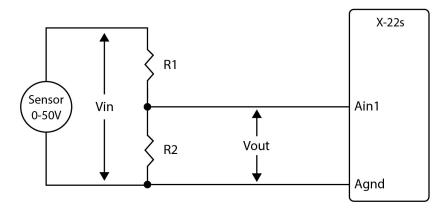
Generally, you can choose a 10K Ohm resistor for R2 and then calculate the value of R1 using the following formula.
