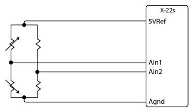
The low input bias and high resolution inputs of the X-22s together with the reference output make the X-22s workable with many bridge sensors without using a preamplifier or other circuitry.
