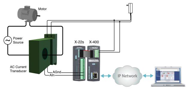
This example uses a current sensor that will measure current up to 20 Amps AC. The sensor produces a linear 0-5VDC output (0V represents 0A and 5V represents 20A) that it can be connected directly to one input of the X-22s analog module. The slope is calculated and entered into the setup pages of the X-400. The slope calculation is given below:
