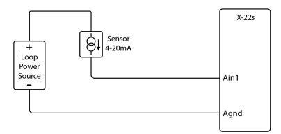
Loop powered current transmitters normally require 7 to 8 Volts across their terminals in order to work properly. The 200-ohm load resistor will drop 4V across the input terminal at 20mA. Allow 2-volts or so for voltage drops across the wiring, especially if the wires are small or long. In this example make certain your loop power source is at least 14-Volts (8+4+2).
